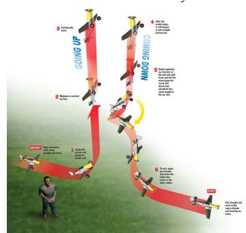
apply either full up-elevator to perform a "wheels down" tailslide, or push full down-elevator to perform a "wheels up" tailslide.
