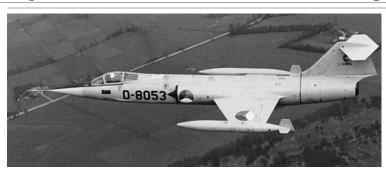
The Lockheed F-104 Starfighter is a single-engine, supersonic interceptor aircraft which was extensively deployed as a fighter-bomber during the Cold War. Created as a day fighter by Lockheed as one of the Century Series of fighter aircraft for the United States Air Force (USAF), it was developed into an all-weather multirole aircraft in the early 1960s and produced by several other nations, seeing widespread service outside the United States.
